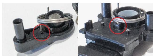
**25.** Place the washer on the small protrusion from the top side of the lever housing.
