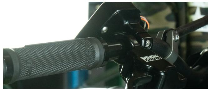
**33.** Ensure the levers and switches are placed evenly on both sides and ensure the angle of levers, switches and bars are as desired.
