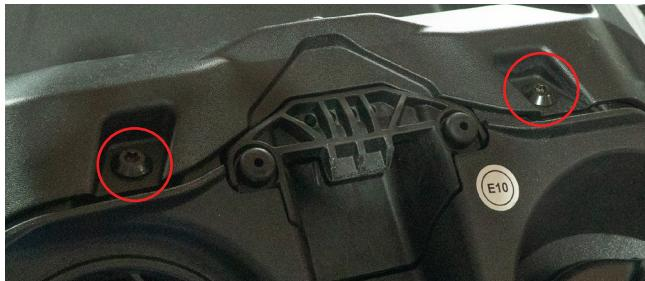
**8.** Undo the two bolts securing the steering clamp retainer piece using a 10mm socket.
