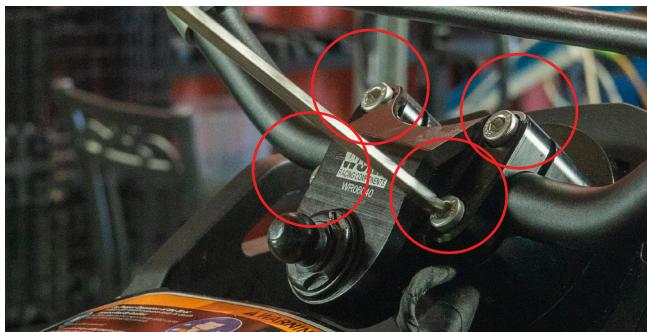
18. Measure the gap between the top and bottom clamp ensuring it is even the whole way around. If not, go back and re-tighten the bolts so the bar is secured evenly.
