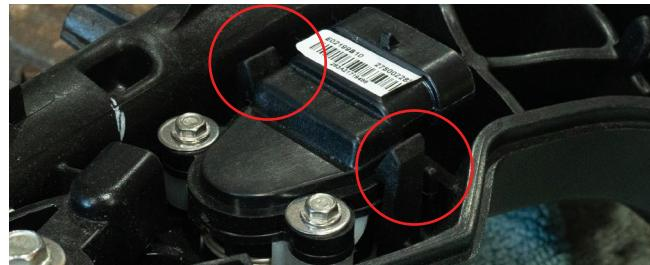
22. To assemble the throttle and IBR assemblies, remove the white spacers from the units.
