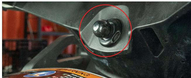
**7.** Open the front storage compartment and unscrew the two torx bolts, pictured below, using a T27 Torx Bit. Remove the dash cover plate by pulling up and away from the ski.
