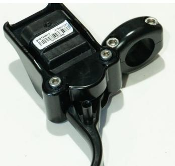
**28.** Clamp the lever housing to the handlebar using a 4mm hex key.
