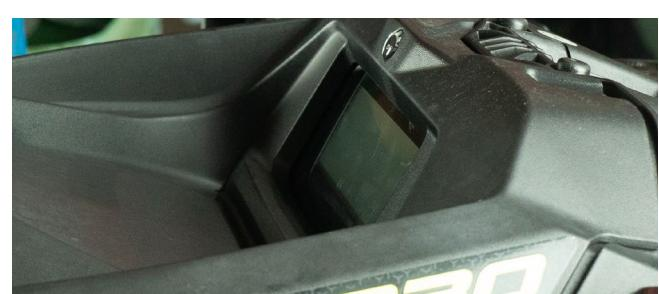
**14.** Secure the DESS post to the top clamp using the OEM plastic lock nut and re-clip the cable to the DESS post.
