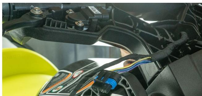
6. Undo the plastic lock nut securing the DESS post in place and unclip the DESS post cable. Retain the lock nut and pull the cable through the back of the steering column.
