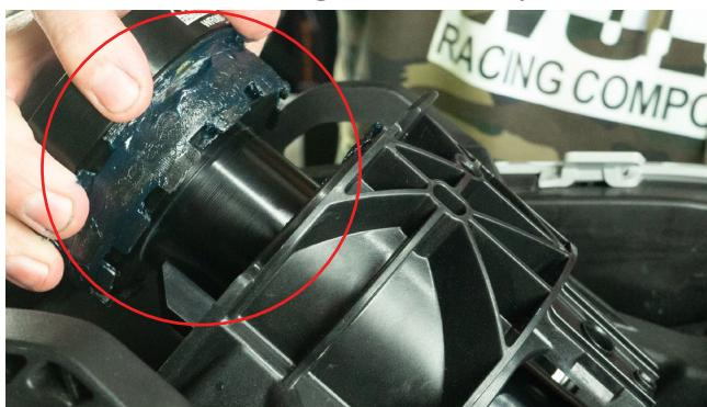
**11.** Slide the steering column back down through the ski, feeding the cables up and through the column, ensuring the worx logo is facing up (as pictured above), with the top steering stoppers facing downwards, and ensure everything fits well.
