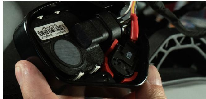
**31.** Secure the back plate of the switch housing using a 3mm and 4mm hex key and the bolts provided.
