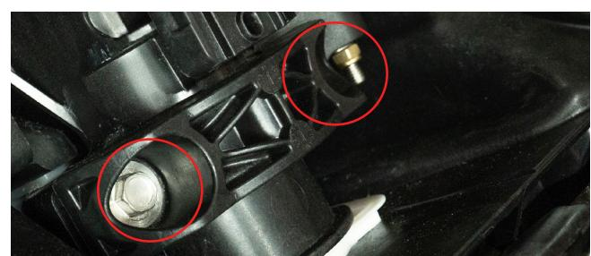
**13.** Re-clip in the dash plate cover and secure using the OEM torx bolts.
