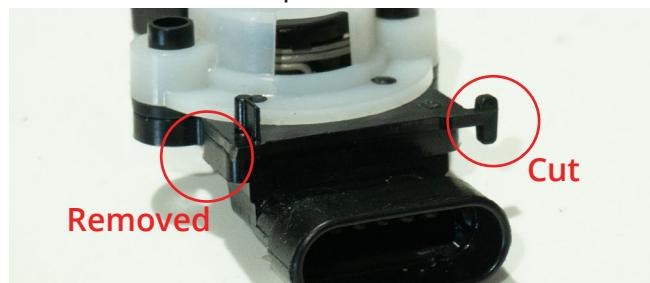
24. If the spring falls away from the unit, replace the locating tabs in the positions show in the images below.
