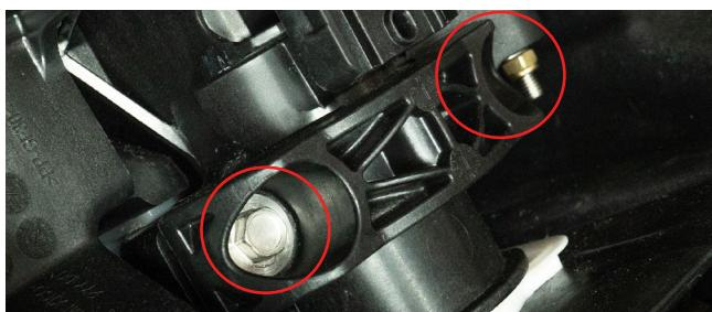
**9.** Pull the steering column up and away from the ski, whilst feeding the cables back through the column as you pull it away.
