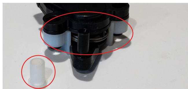
23. Cut the tabs on the outside of the actuators as pictured below.
